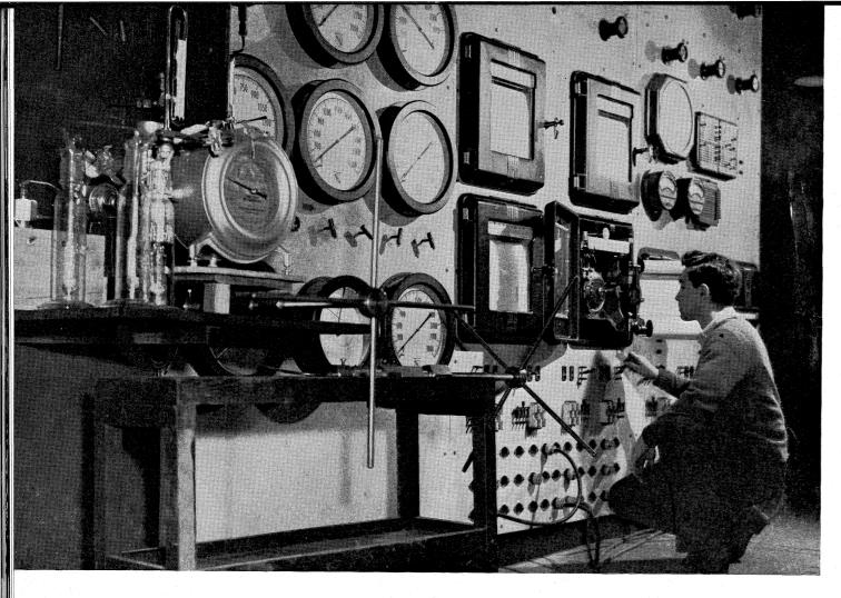
THE University's high-pressure research laboratory was one of the first in the country when it was built in 1926. Out of it have come many useful discoveries in chemical engineering, such as the process for making acetic acid by reacting carbon monoxide and methanol at high pressure. Studies can be made at gas pressures as high as a thousand atmospheres - 15,000 pounds per square inch.
