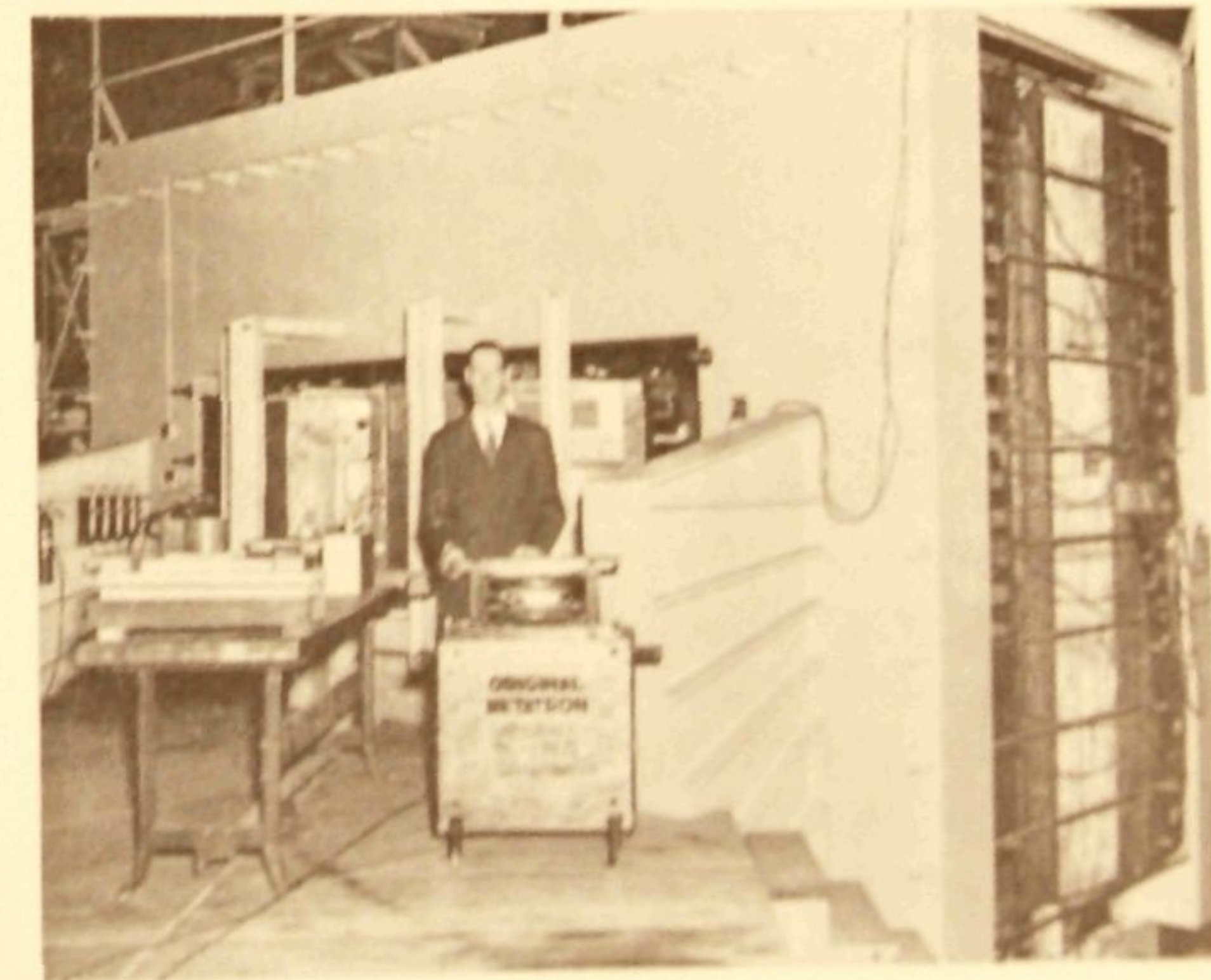
THE BETATRON, NOW WIDELY USED IN NUCLEAR RESEARCH, INDUSTRIAL RADIOGRAPHY AND CANCER TREATMENT, WAS INVENTED AT THE UNIVERSITY IN 1940 BY PROF. DONALD W. KERST.
