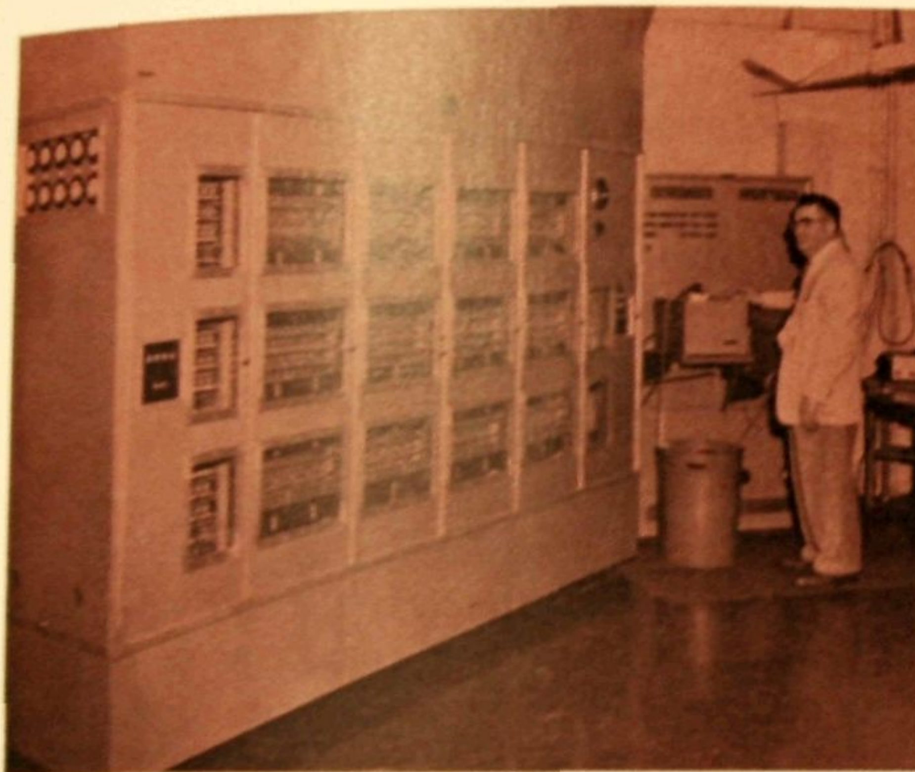
DATA-PROCESSING IN MUCH RESEARCH IS SPED BY ILLIAC, A HIGH-SPEED DIGITAL COMPUTER, DESIGNED AND BUILT ON CAMPUS.
