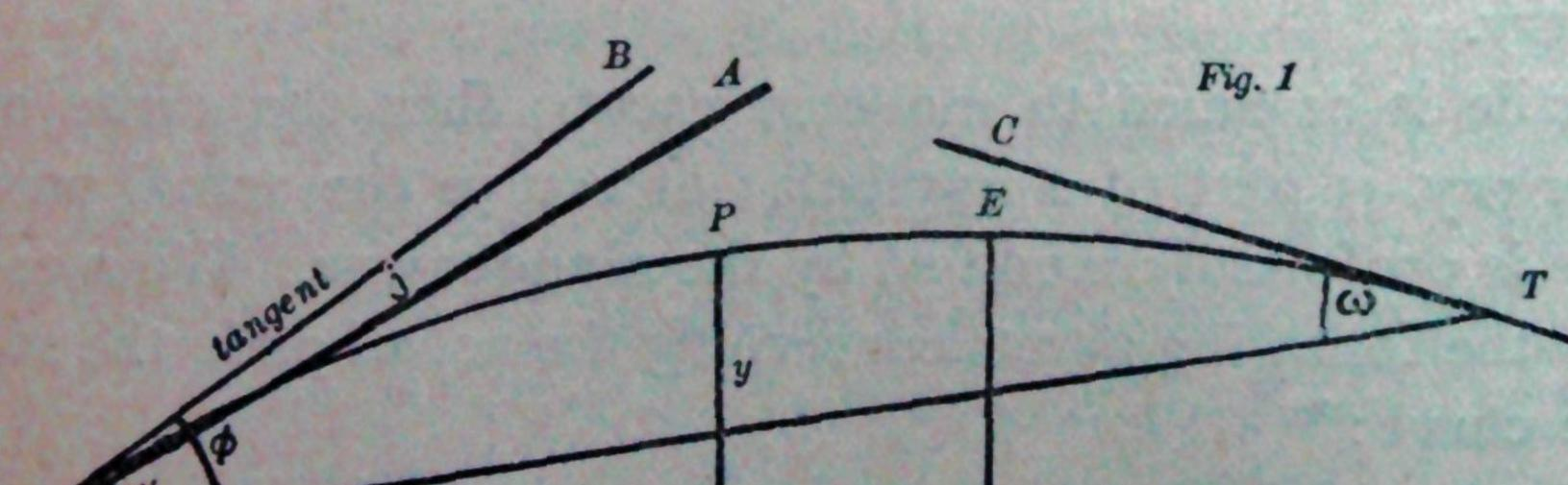
Let G in Fig. 1 be the gun (more accurately the muzzle of the gun), T the target, GN a horizontal line, GB a tangent to the curve at G; then
