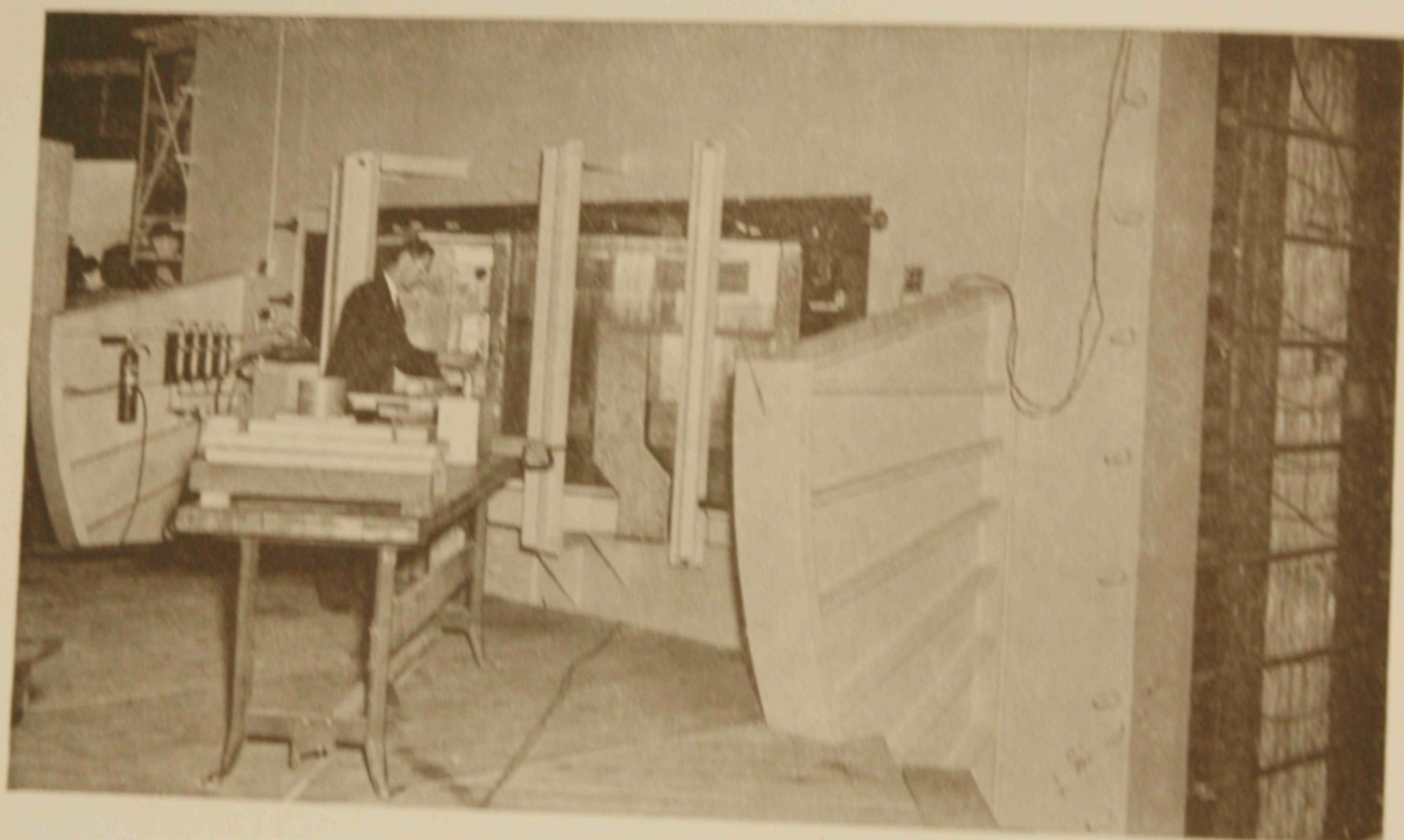
The world's biggest betatron, completed in 1950, produces 340-million volts and enables University physicists to carry on nuclear physics research impossible elsewhere.
